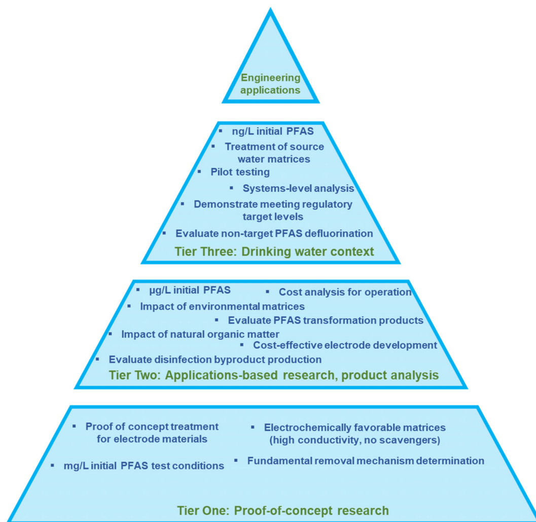
FIGURE 4 Summary of research needs for implementation of electrochemical treatment for per- and polyfluoroalkyl substances (PFAS) mitigation in drinking water. Each tier represents a different foundation of research that needs to be examined in order to progress to the goal of engineering application. Tier one research focuses on proof-of-concept research to verify that a technology can work for a specific contaminant. Tier two research focuses on assessing different applications of research and the influence of matrix factors, transformation products, and the costs associated with treatment. Tier three focuses on research explicitly focused on implementation for drinking water treatment and includes studying the impact of environmentally relevant conditions and is validated based on regulatory targets. Finally, the peak of the pyramid is “engineering application” which requires a stable foundation supported by the underlying tiers of research
